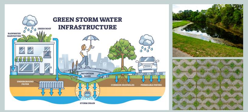
Photos and images above depicting types of green stormwater infrastructure, which includes rainwater harvesting, rain gardens, planter boxes, green roofs, bioswales, permeable pavements, green streets and alleys, green parking, urban tree canopy, and land conservation. The top right image depicts a bioswale. The bottom right image depicts permeable pavement.
